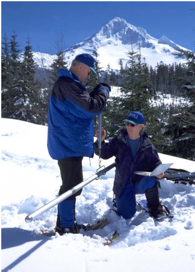
Left: Data collectors are weighing the snow to determine the amount of water content in the snowpack. It is converted to water inches and is compared to 30 year average to determine percent of average snowpack.
