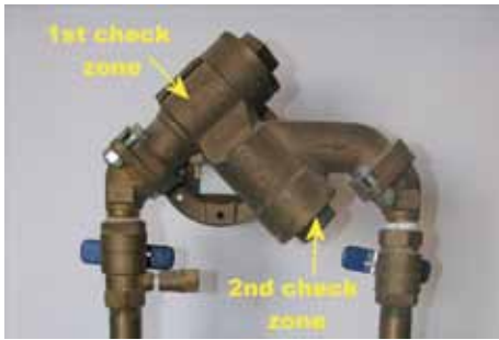
Figure 5: Open test cocks (1st check zone) and remove the check cap (2nd check zone).
