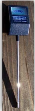
Figure 1. Although somewhat inaccurate, a houseplant water meter is a tool to evaluate water needs in the garden.
