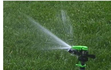
Figure 8. Gear-driven heads use the flowing water to turn a series of gears that rotate the head. Gear-driven heads are quieter to operate than impact heads.
