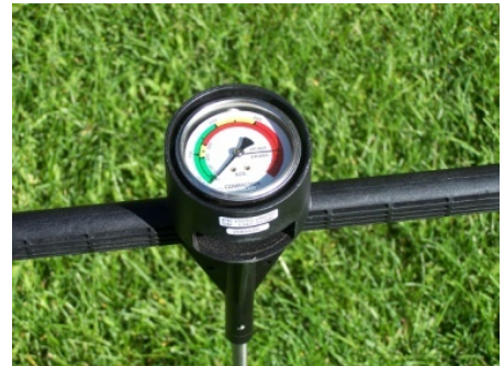
Figure 9. Soil penetrometer measures the pressure it takes to push the probe into the soil. It is a great tool to evaluate soil compaction.
